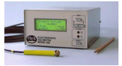
The Trek Model 542 Electrostatic Voltmeter provides accurate noncontacting measurements of electrostatic surface voltage associated with EOS/ESD sensitive processes. The microprocessor based Model 542 is ideally suited to monitor critical operations associated with semiconductor, LCD, electronic assembly, and other processes where static charge accumulation poses a threat to production yields or product quality.
